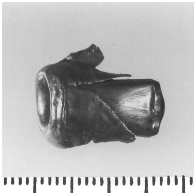
Fig. 6 Nosler bullet recovered in the cotton wool filled butt after penetration of 50 mm thick wood. The nose ( left ) is destroyed, and the jacket peeled back
